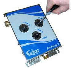
**◄2**Remove valve knobs and set tools aside.
