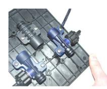
**<2**To remove the Venturi procede as shown
