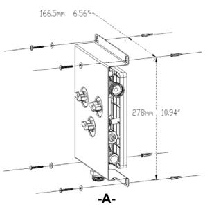
Fit the unit on the wall using the supplied wall anchors
